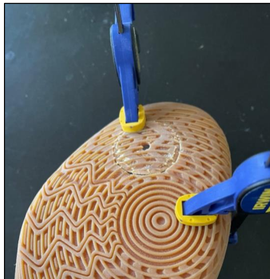
Figure 15. Adhering midsole to outsole
