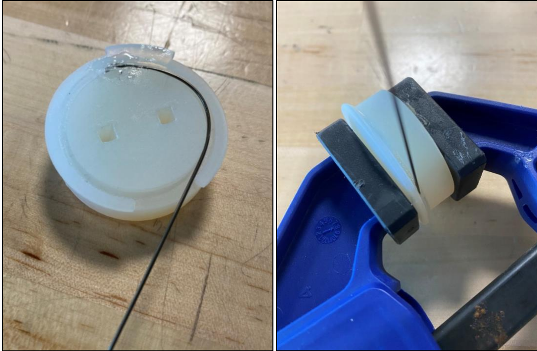
Figure 12. Construction of rotating mechanism with epoxy
