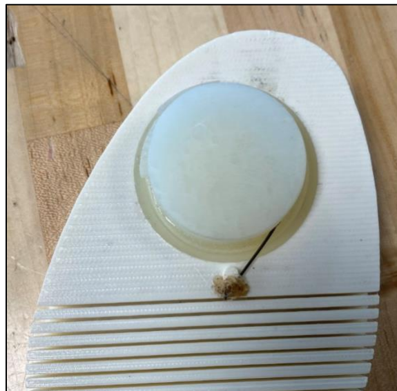
Figure 13. Anchoring of nitinol to midsole
