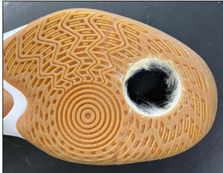
Figure 14. Rotating mechanism hole in outsole
