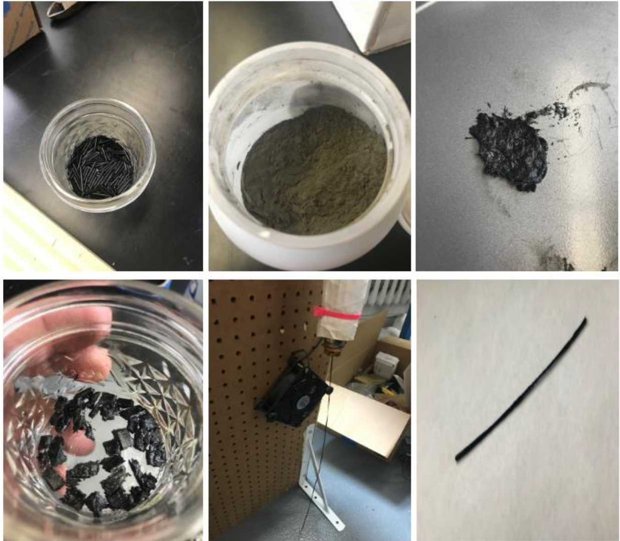
Figure 4.2: i: PA12 pellets pre-dissociation, ii: NdFeB powder iii: NdFeB/PA12 mixture, iv: pelletized NdFeB/PA12, v: NdFeB/PA12 being extruded, vi: final NdFeB/PA12 filament
