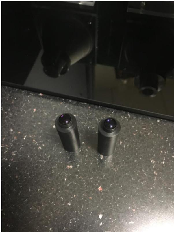
Figure 19: Lens for liquid light guide
