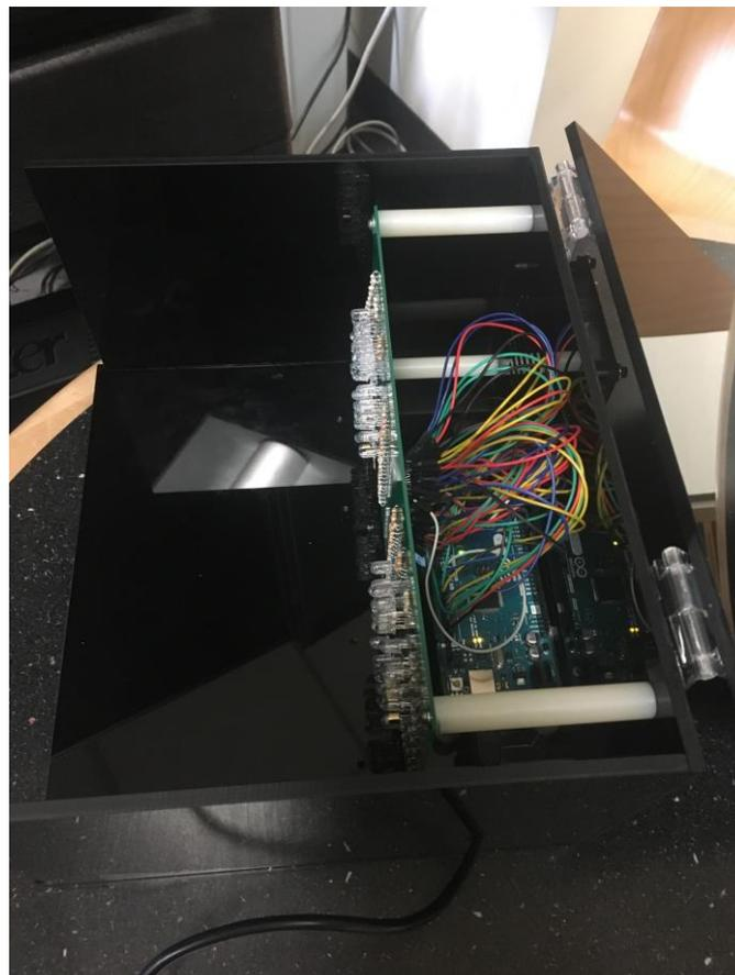
Figure 17: LEDs and Arduino board
