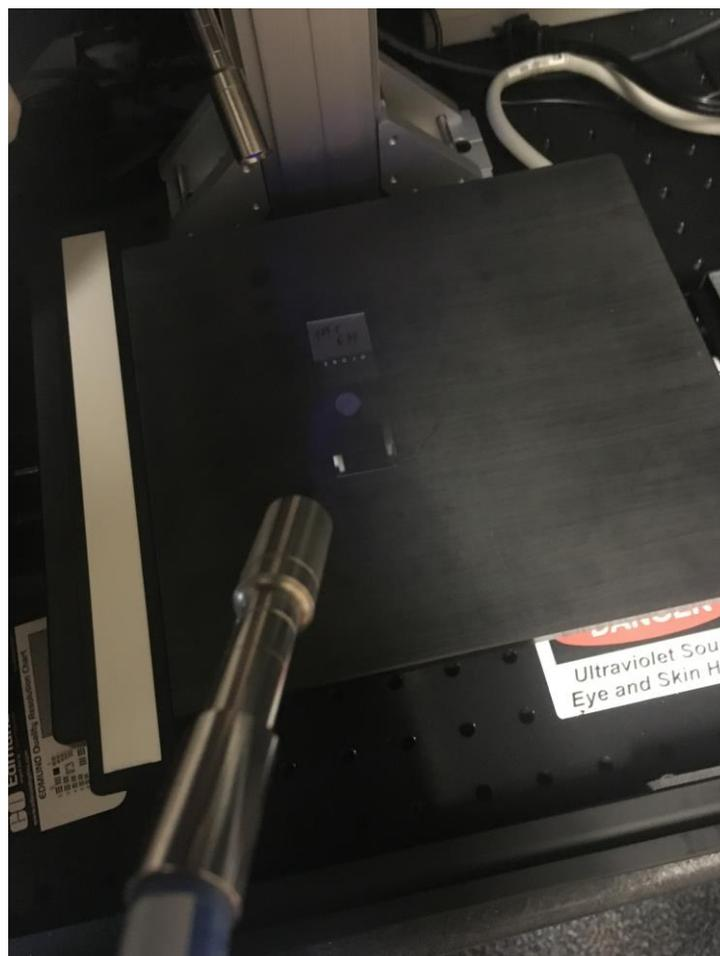
Figure 27: Projection of light from liquid light guide
