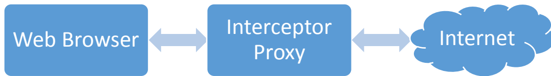
Figure 5 - Interaction with the proxy server. HTTP requests are made through the web browser, redirected to the proxy, recorded, and forwarded to the Internet. Responses from the internet are directed to the proxy, recorded, and forwarded to the browser.
