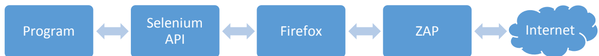
Figure 6 - The basic representation of the flow of commands when using the data collection tool.
