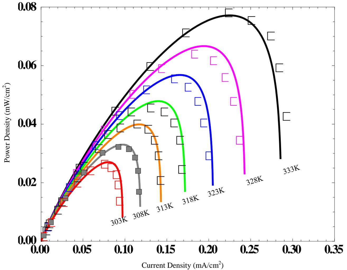
Figure 40: Power Curve, 1.0M, variable T [36]
