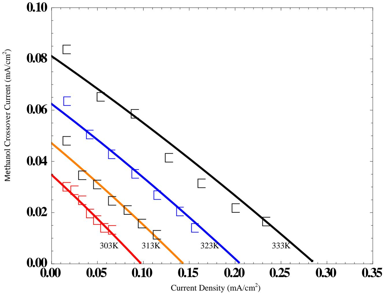
Figure 41: Methanol Crossover Current Density versus Current Density, 1.0M, variable T [36]
