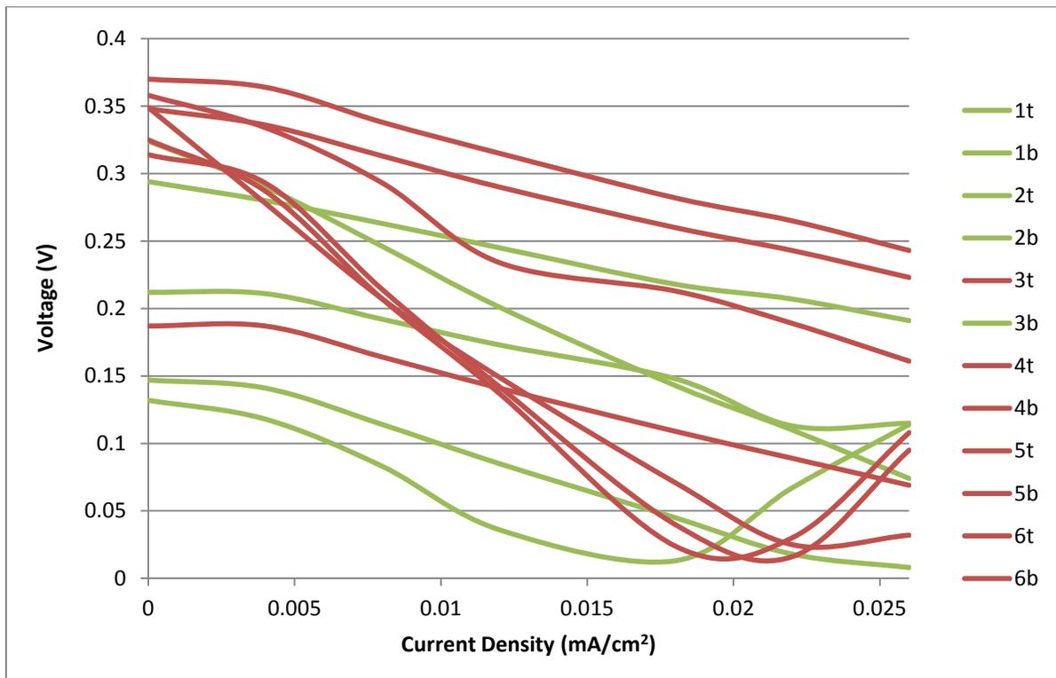
Figure 29: Individual MEA Performance by Manufacturer (Stack Layout, MeOH Gel Fuel)
