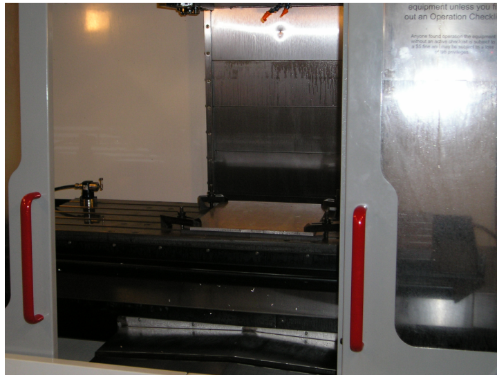
Figure 17: Aluminum Stock clamped in CNC
