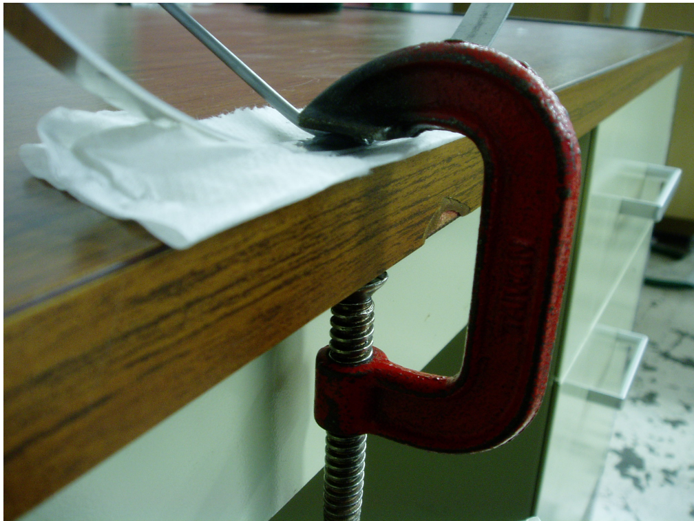
Figure 13: Clamp securing rod to ring connection
