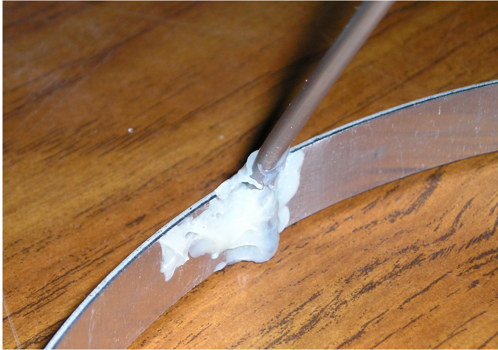
Figure 14: Rod epoxy connection to ring
