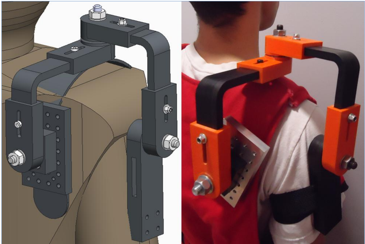
Figure 43—Mechanism and torso mount subsystems together in final design, conceptual (left) and prototype (right)
