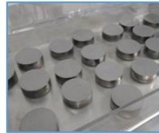
30mm OD pellets pressed at 200 MPa
