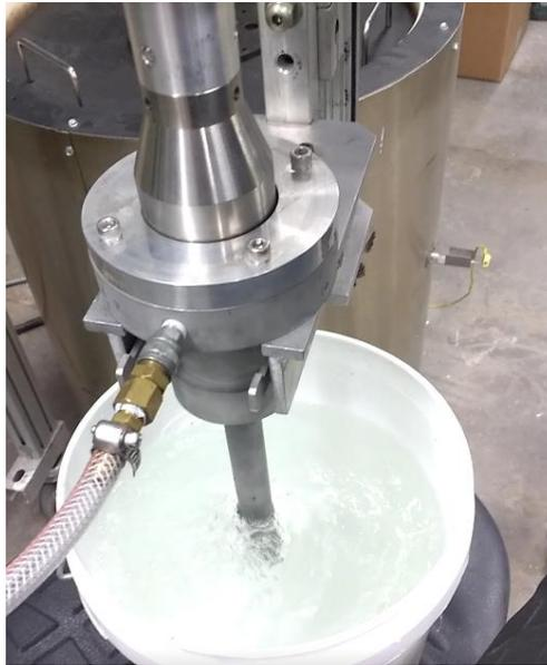
*Figure 5: ultrasonic degasser used before casting of ISGR and SHS material, demonstrated in water.*
