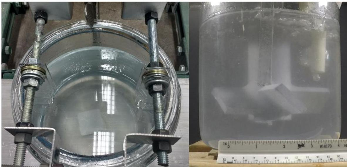
*Figure 13: mixing setup showing position baffles and gas insertion tube in glycerin/water mixing tank. Impeller height was set to 1in. from the tank bottom, and tube height 0.75" from the upper edge of the impeller blades.*
