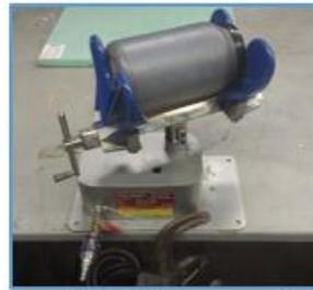
CuO added, then paint shaker mixing to avoid fire hazard
