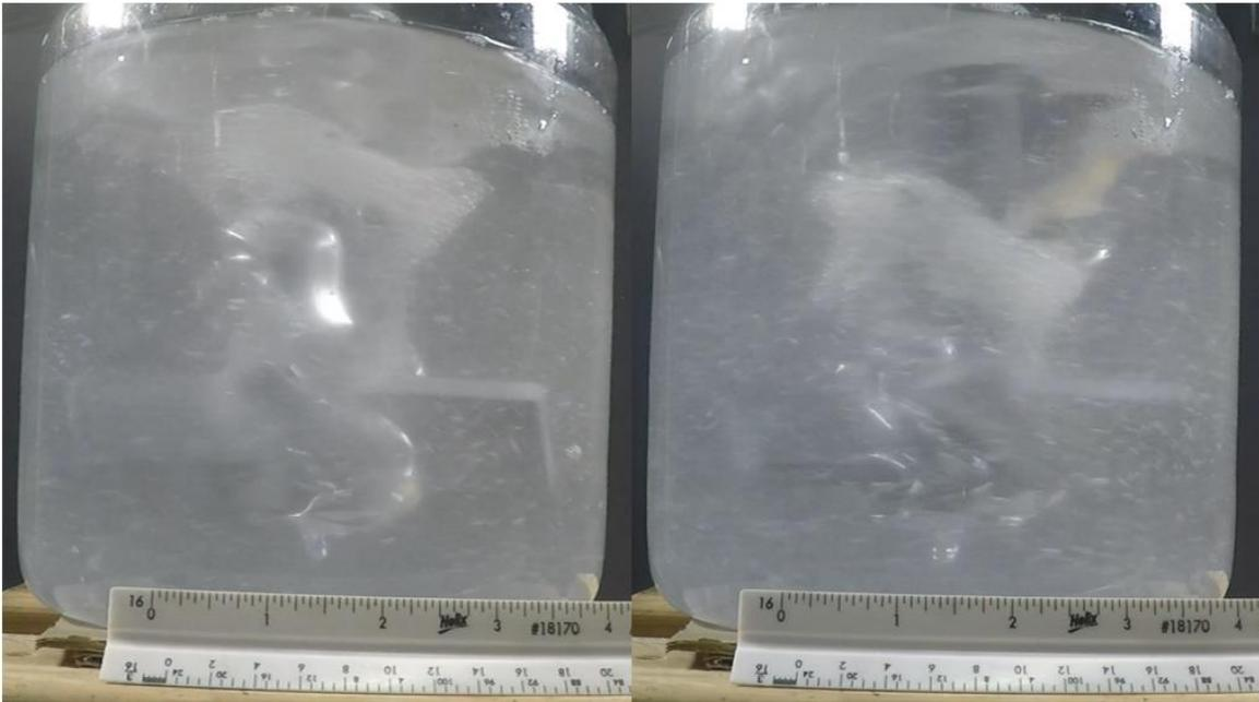
*Figure 23: unbaffled mixing test, 200 and 250RPM*
