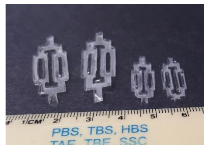
Figure 41: Gelatin structures made with Shrinky-Dink derived mold
