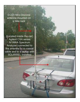
**Fig. 4.2** A photograph of the mobile wireless spectrum measurement testbed employed in this research. Components of the testbed include a mini-discone/ridged-horn antenna, a spectrum analyzer and a laptop with SQUIR-REL installed.
