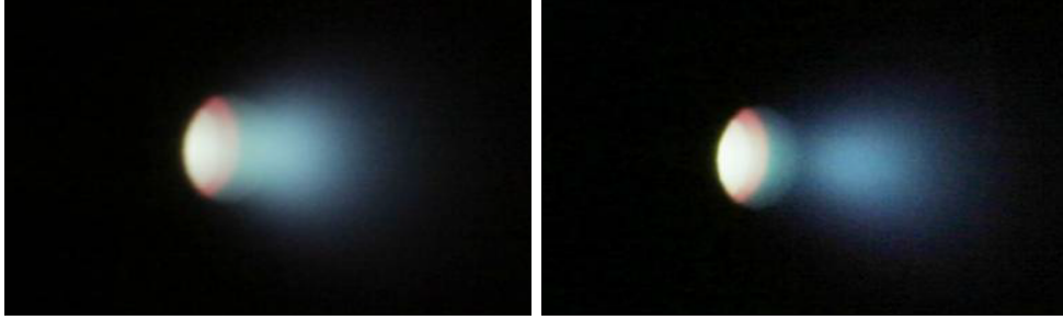
Figure 6: Cathode Spot at 5.5 sccm (left) and 10 sccm (right) 3
