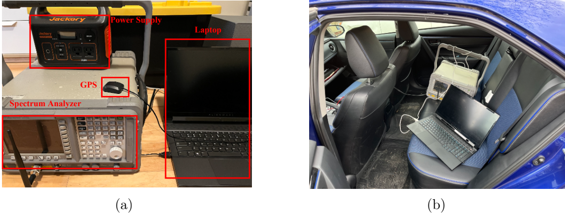
Figure 5-1: Data collection platform, (a) different components of the data collection platform (b) platform during the data collection with a moving vehicle
