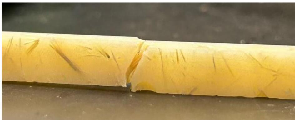
**Figure C5. Bamboo fiber 3 wt. % tensile fracture side view**
