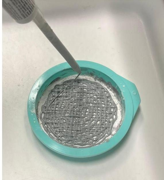
**Figure 7.** Trial composite using a high-viscosity epoxy that proved difficult to work with
