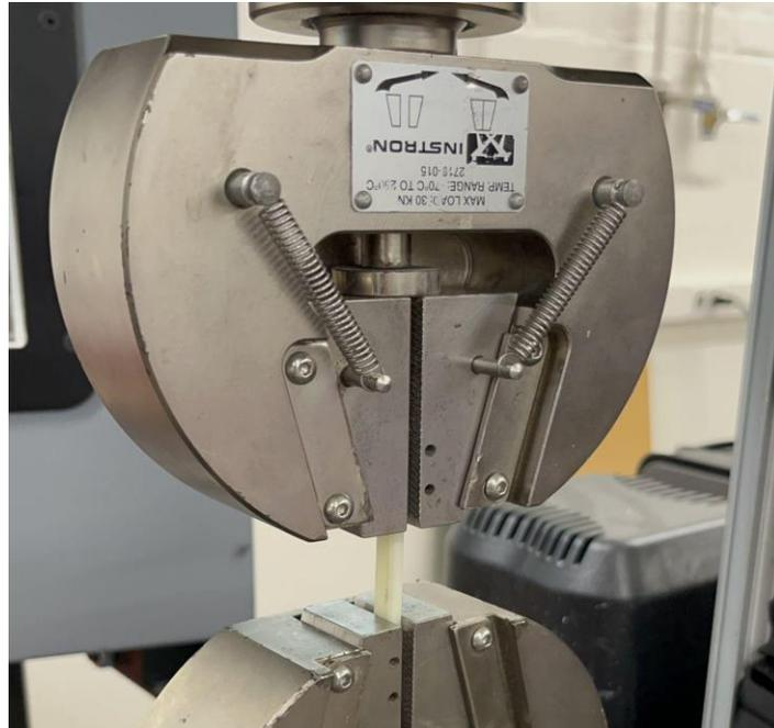
**Figure 11.** Instron 5567A tensile testing apparatus using claw grips
