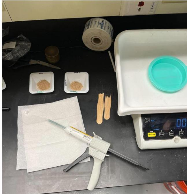
**Figure C1. Materials used for creating a CELF fiber composite**
