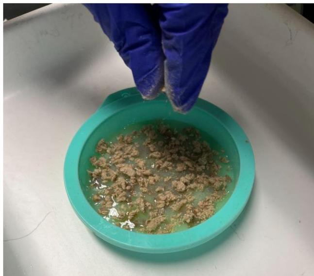
**Figure C2. Placing CELF fiber clumps into the mold during the sample-making process**
