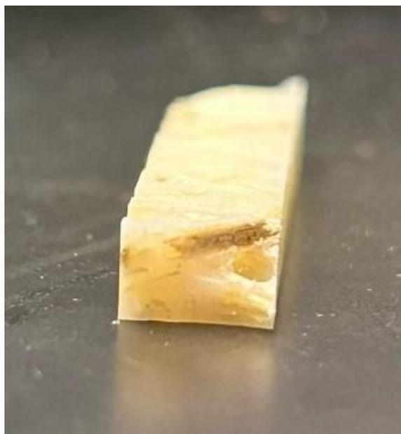
**Figure C6. Bamboo fiber 4 wt. % tensile fracture cross-section**
