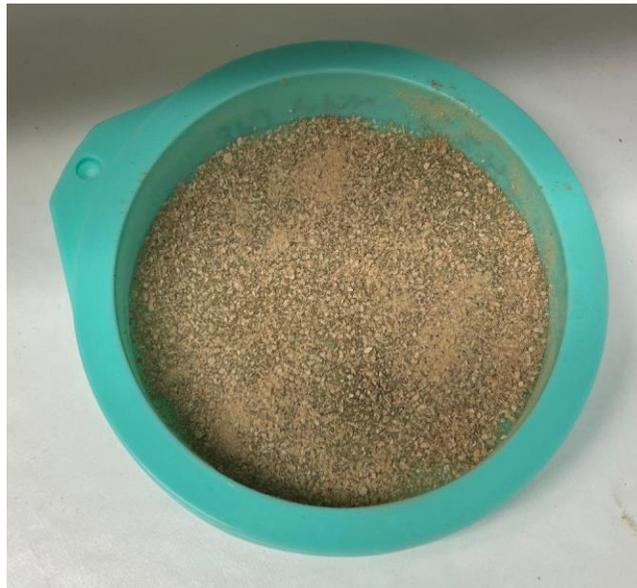
**Figure 8.** Ball-milled CELF layer atop epoxy layer of 2 wt. % composite sample
