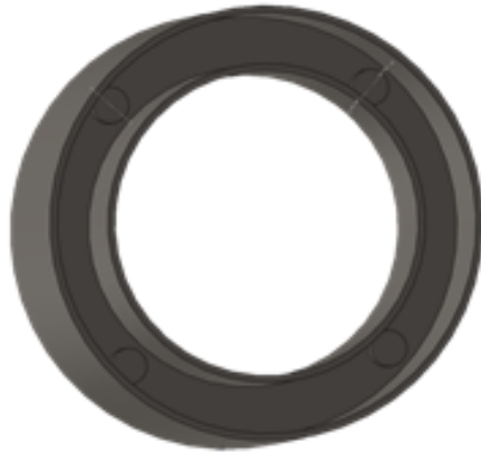
Figure 36. Solidworks model of housing (no springs)
