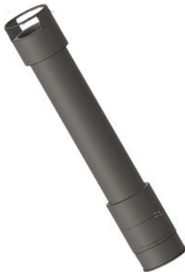
Figure 33. Solidworks model of modified, spring loaded middle insert
