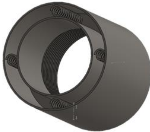
Figure 37. Solidworks model of housing (with springs)
