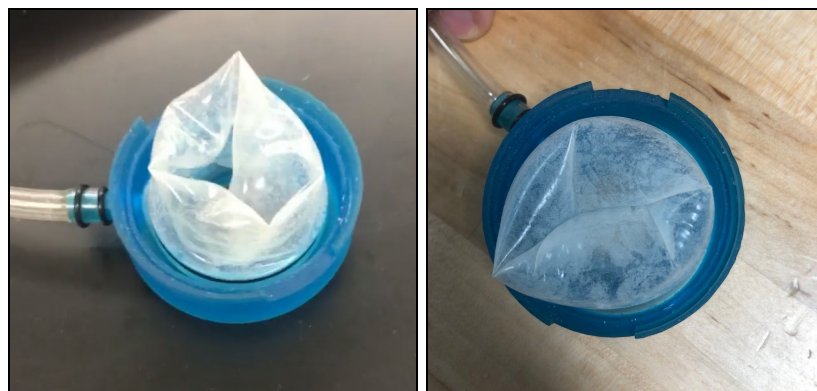
Fig. 28. Inflatable Seal Pre and Post Inflation
