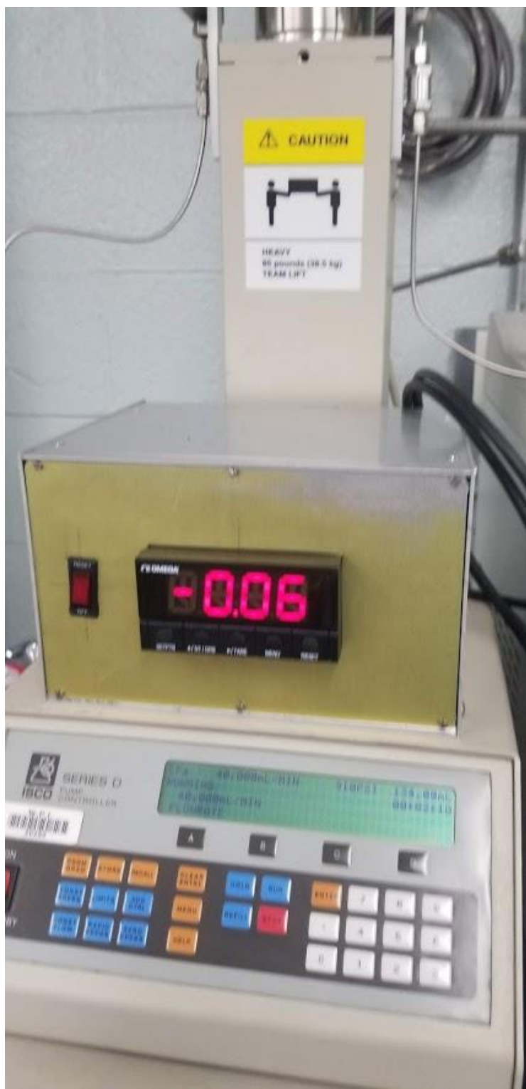
Figure A4: Pump controller and pressure transducer displays. Note system PSI indicator on pump controller.
