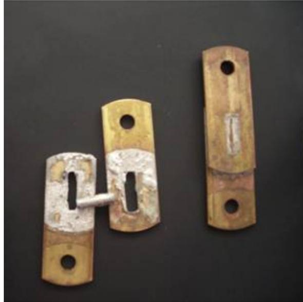
**Figure 2-4 Riley Air Link (70°C Activation) Activated (left) and Un-activated (right)**
