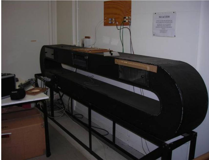
**Figure 3-11 Plunge Test and Ramp Test Apparatus**
