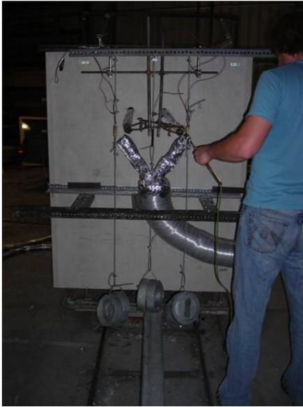
**Figure 3-13 Measuring Simulated Wind Speeds**
