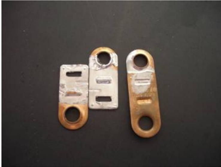
**Figure 2-6 Globe Technologies Model K Link (57°C Activation) Activated (left) and Un-activated (right)**
