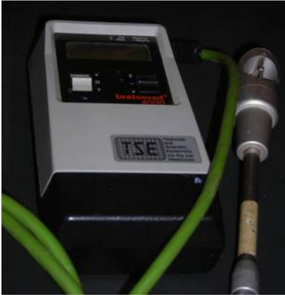
**Figure 3-14 Handheld Anemometer used for Velocity Measurements**
