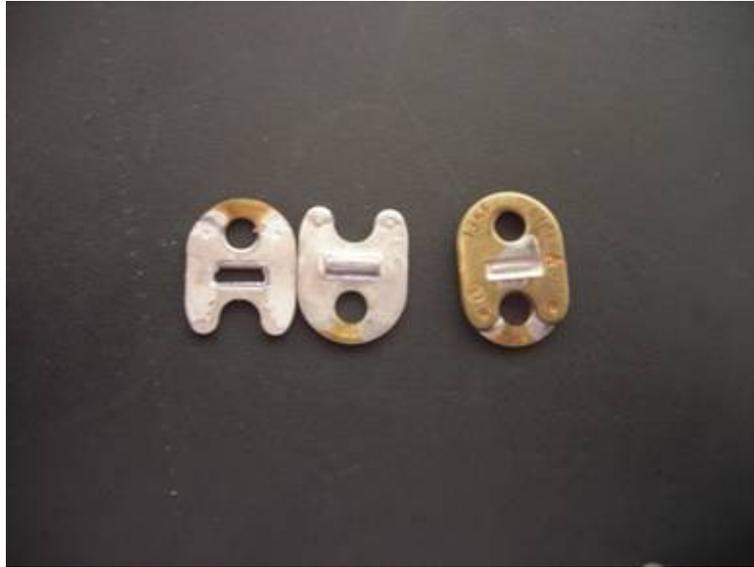
**Figure 2-5 Globe Technologies Model A Link (57°C Activation) Activated (left) and Un-activated (right)**
