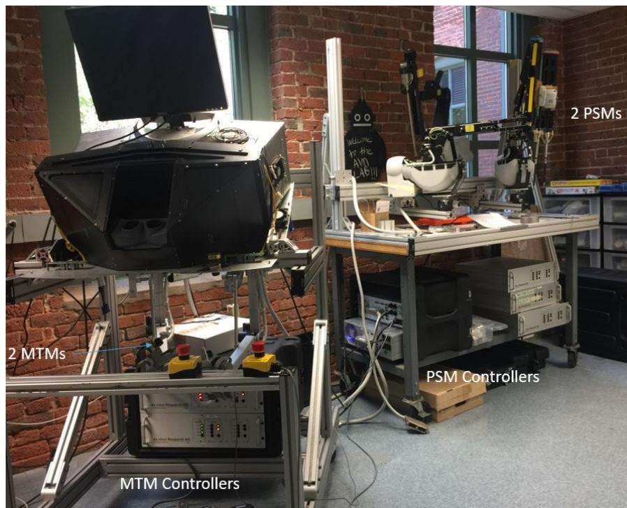
Figure 3.4: da Vinci Research Kit Hardware at Automated and Interventional Medicinal Laboratory
