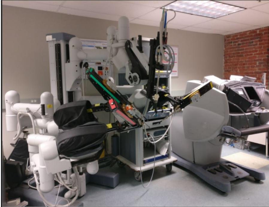
Figure 3.1: The da Vinci Surgical System at Automated and Interventional Medicinal Laboratory
