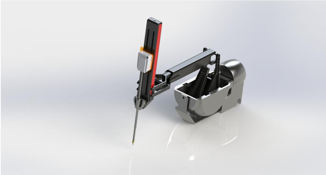
Figure 6.1: Patient Side Manipulator Solidworks Model
