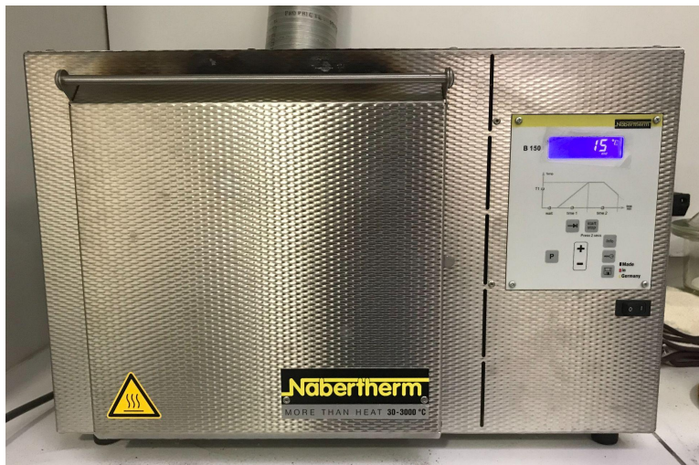
Figure 9. Nabertherm oven used for loss by ignition
