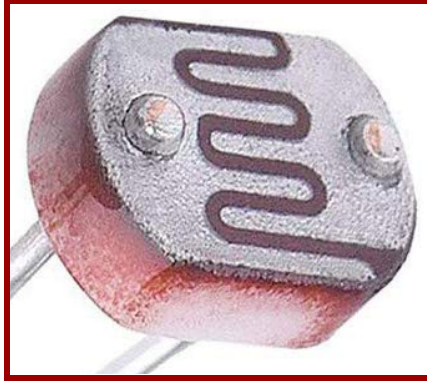
Figure 20: The Reactive Head of a Photoresistor [47]
