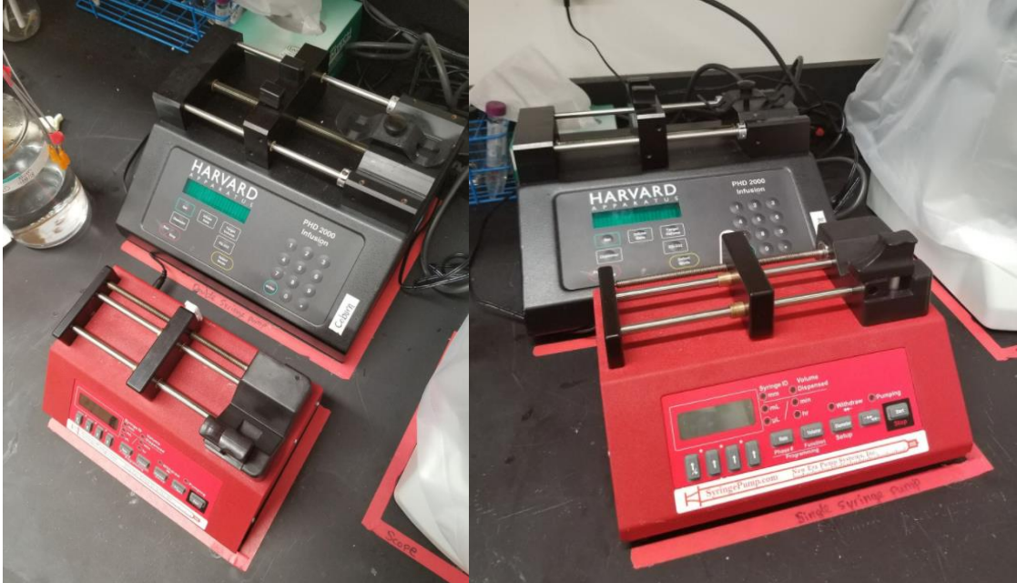
Figure 3: The syringe pumps placed on the aligned to the marked red tape. The single syringe pump (red) is meant for the dispersed phase and the double syringe pump (black) is meant for the continuous phase
