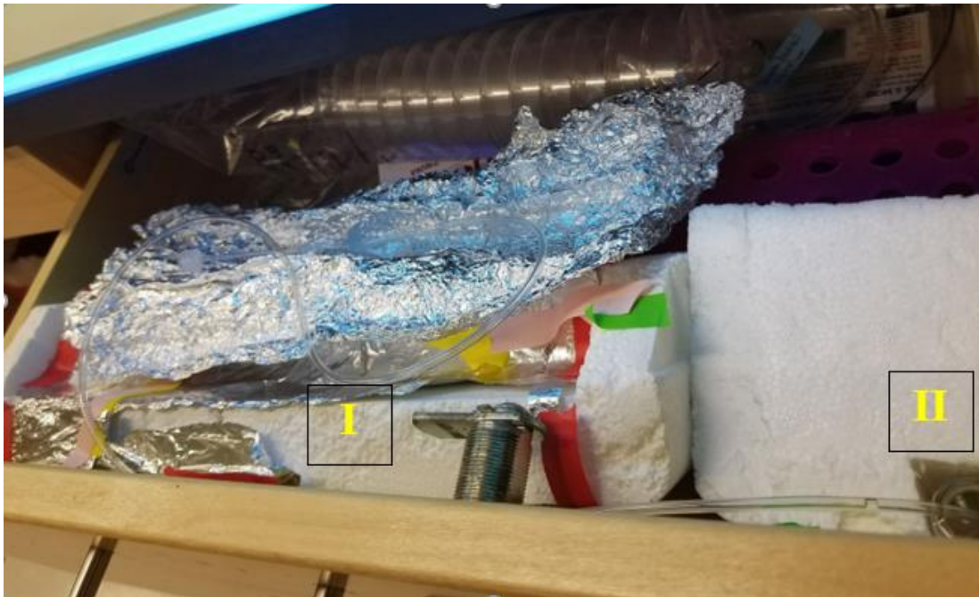
Figure 5: Setting up of the (I) V-boat and (II) collecting vial in the drawer with the UV light bulb above it. An extra sheet of aluminum foil is on the top which can be moved in placed to protect the contents of the drawer other than the setup from UV exposure
