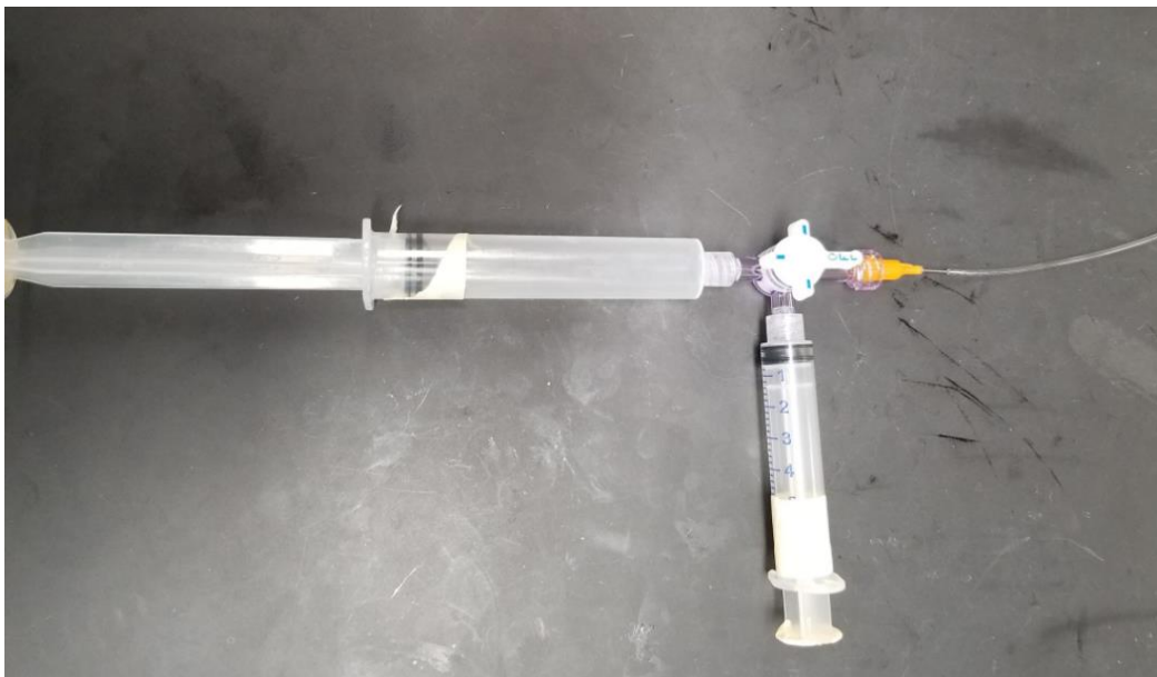
Figure 6.1: Syringe Stopcock Complex. The Three-way stopcock connected to the 10-mL syringe (left), the 5-mL syringe (bottom) and the Tygon™ tubing via the Luer Lock and hypotube needle (right)
