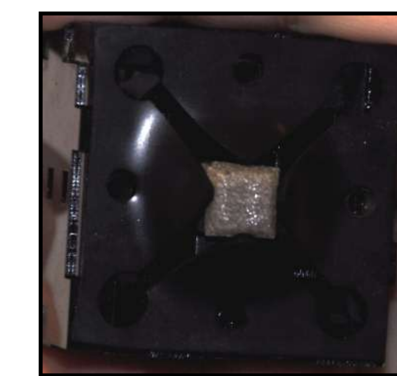
A 10 mm tile coming through a diaphragm test rig.
