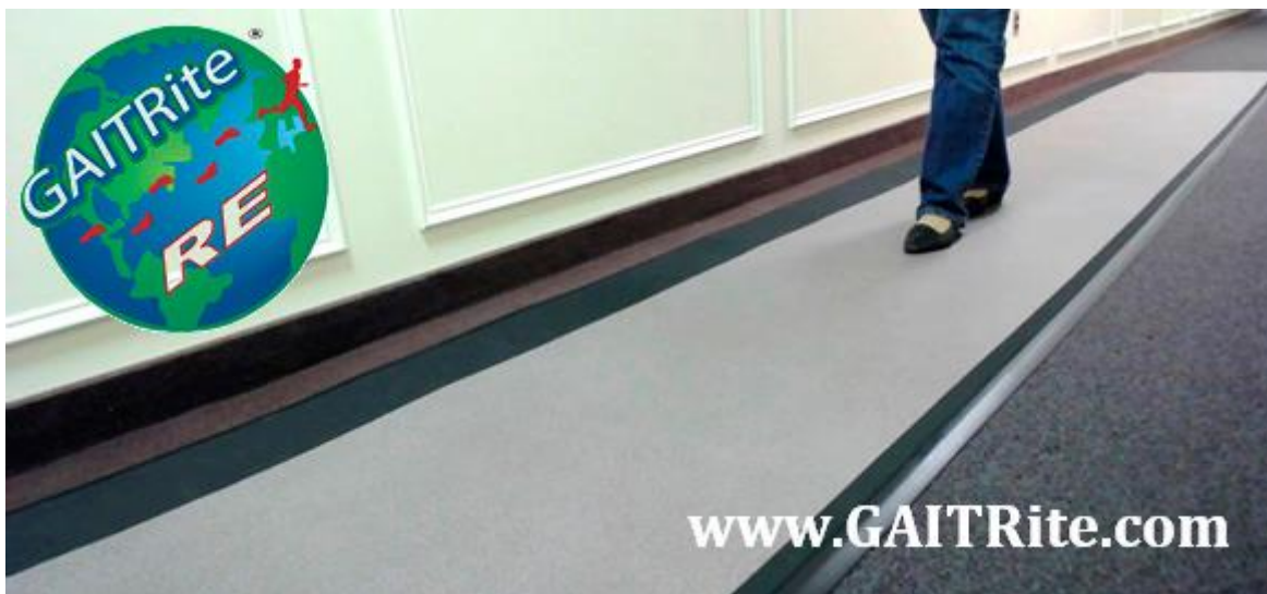
Figure 7: GAITRite Force Sensing Carpet [31]
