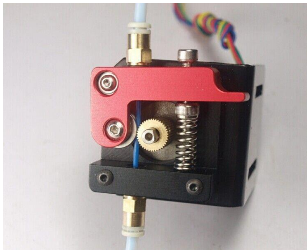
Figure 8: Open extruder to show the filament and its interaction with the drive gear and idler (Unknown)
