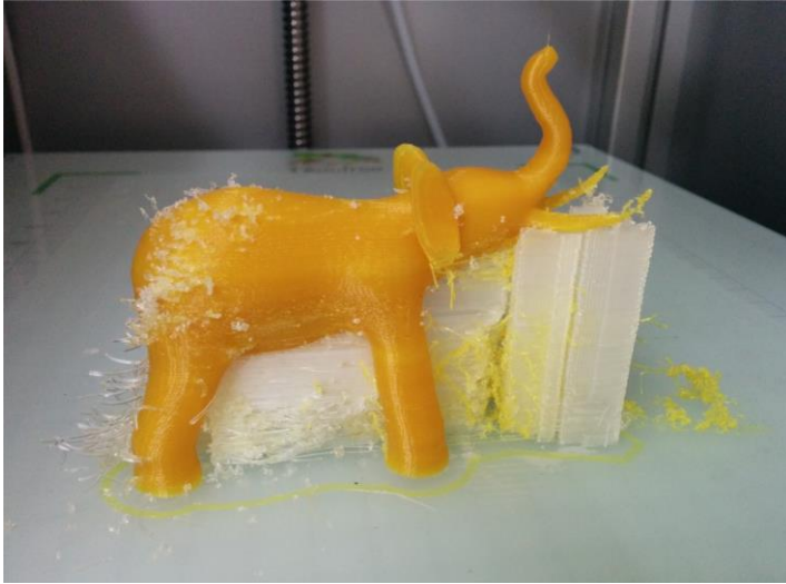
Figure 12 (left): Oozing left on the surface of a finished print (Nick Lievendag, 2014)
