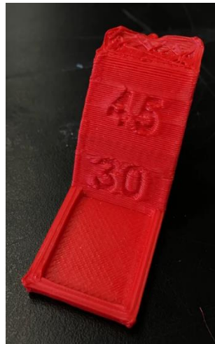
Figure 35: Failed initial overhang test print
