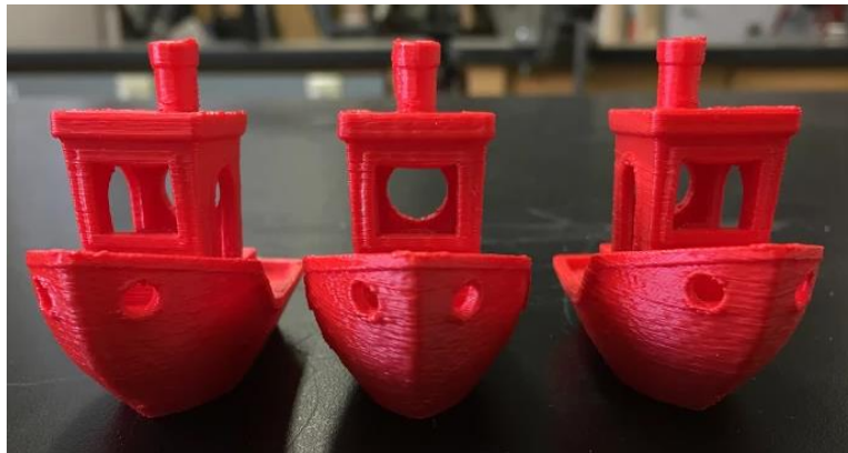
Figure 41: Front view of successful 3DBenchy test prints
