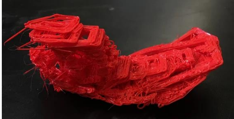
Figure 40: Failed print due to poor bed adhesion, causing layer shifting
