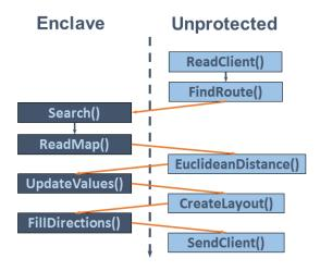
Figure 23: ECALL/OCALL Interfaces without Reduction
