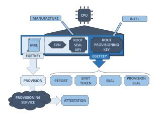
Figure 7: Key derivation process.
