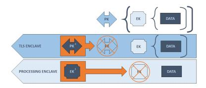
Figure 12: Data Protection Through Multiple Enclaves.
