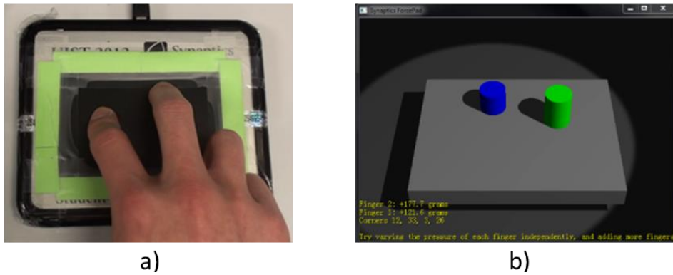
Figure 1: ForcePad (a) and visualization tool (b). It can provide 3D touch information including 2D touch position and 1D pressure with 6-bit resolution and 1000g force, for up to five fingers.
