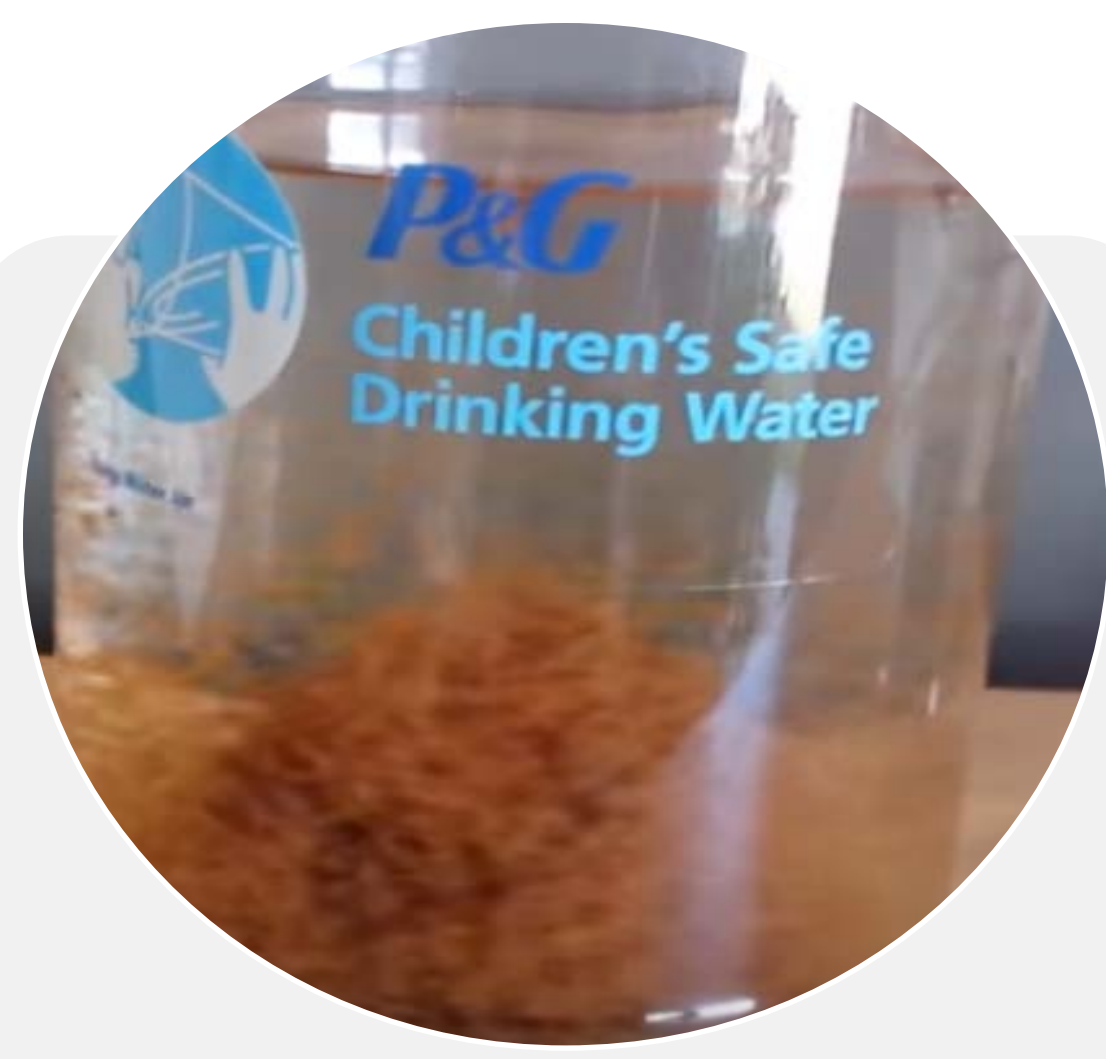
P&G Packet Settling Sediment
