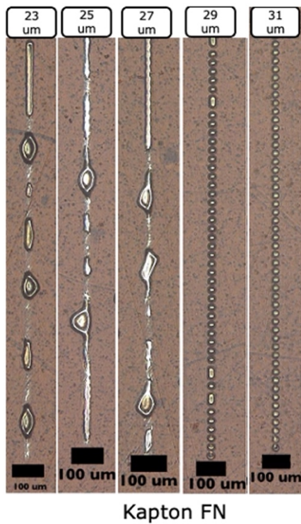
Figure 39. 1 pixel-wide traces printed on Kapton FN with drop spacing from 23 \mu\text{m} to 31 \mu\text{m} .
