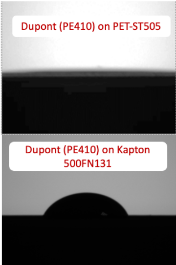
Figure 11. Goniometer images for the smallest and largest contact angles.
