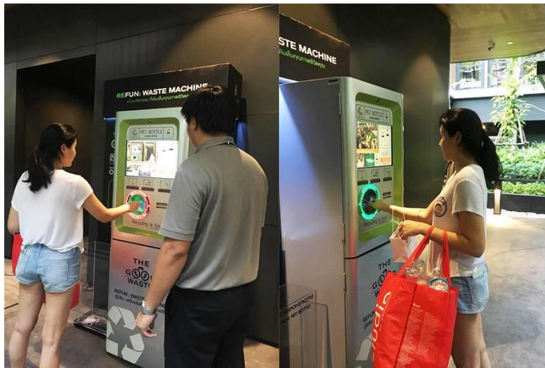
Figure 6. Refun Machine. The Refun Machine in use, collecting plastic recyclables in exchange for money.
