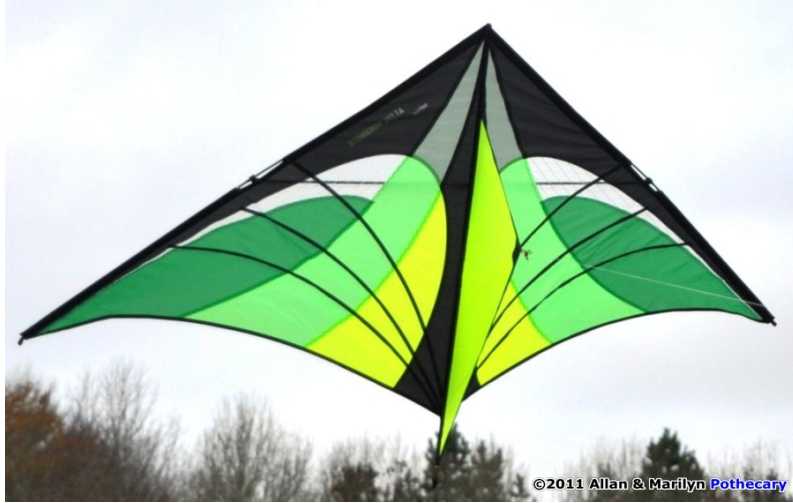
Figure 2.14: A delta style kite. Delta style kites can be configured to fly at high angles, allowing them to be flown in laterally constrained locations [5].
