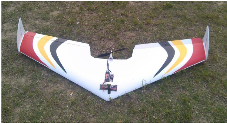
Figure 2.16: A fixed-wing RC aircraft. This is a flying wing style craft with a rear propeller. Its flight would be greatly hindered by any protrusion of the mounting system [7].
