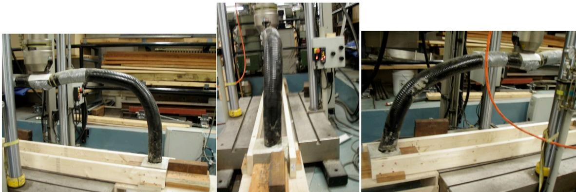
Figure 37 - Arch 4 Failure
