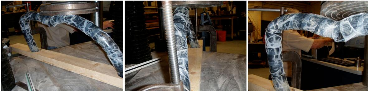
Figure 45 - Mini Arch 1 Failure
