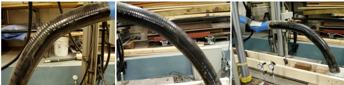
Figure 41 - Arch 5 Failure
