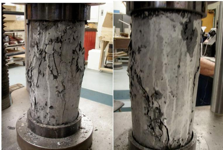
Figure 19 - Results of Cylinder Sample 2 Compression Test
