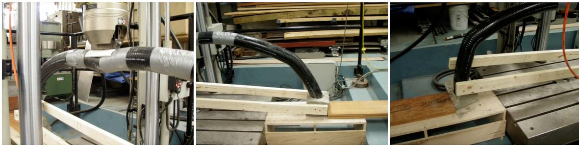
Figure 27 - Arch 1 Failure
