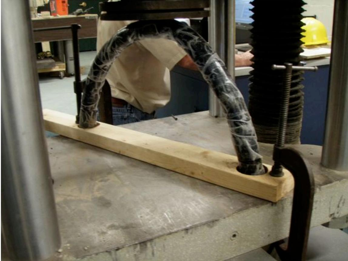
Figure 16 - Mini Arch Test Setup
