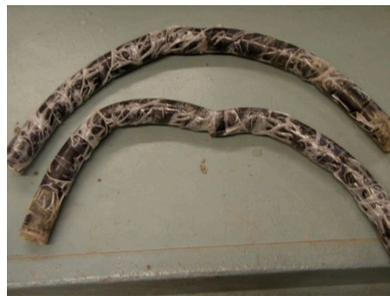
Figure 48 - Mini Arch Failure
