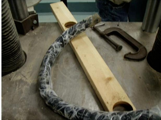
Figure 10 - Mini Arch Test Restraint
