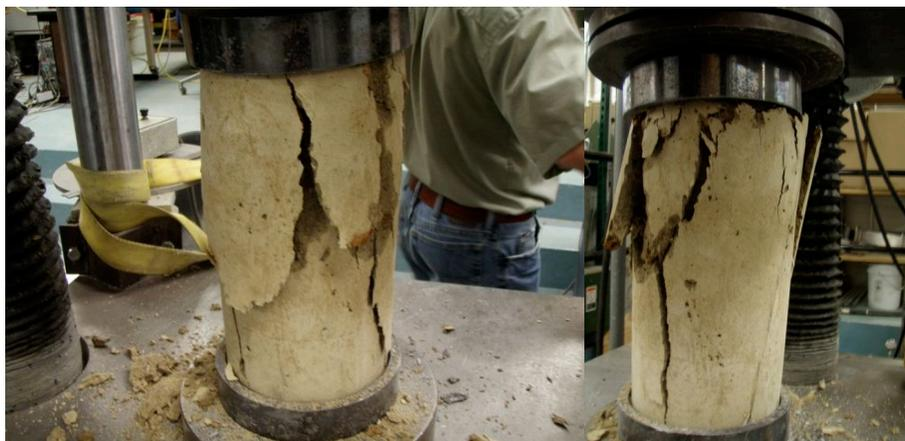
**Figure 21 - Cylinder Sample 3 Compression Test Results**
