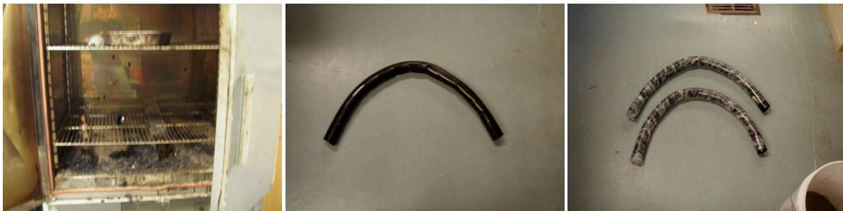
**Figure 8 - Mini Arch Bending Process**
