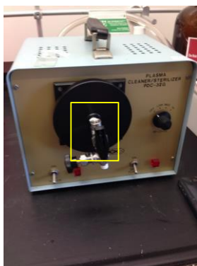
Figure 5E: Open exhaust valve (highlighted in yellow) while holding the door to release vacuum
