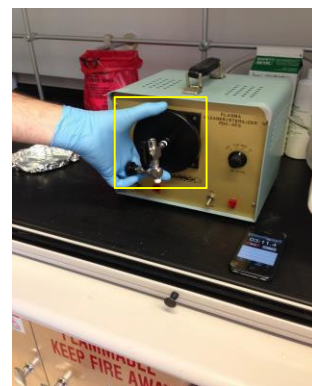
Figure 5B: Hold the round metal door to the vacuum chamber
