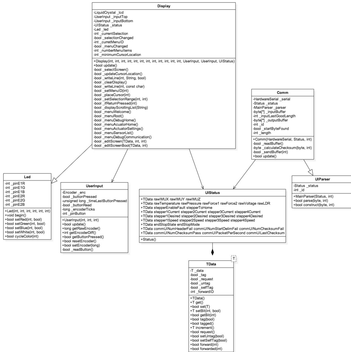
Figure 6-3: UML class diagram for UI Code V1.
