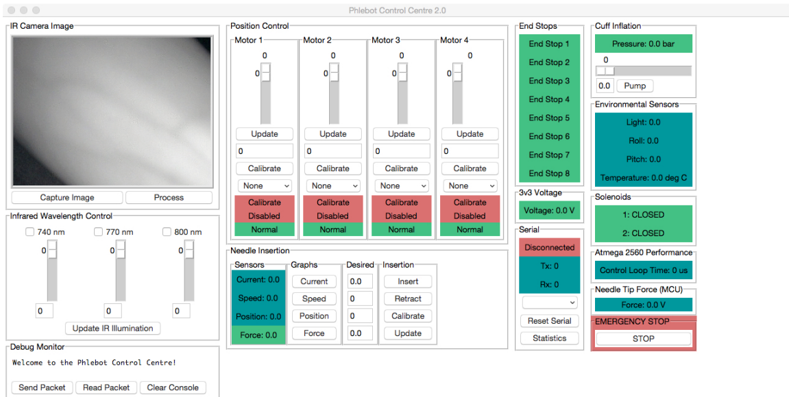
Figure 6-8: Phlebot Control Center V3 with Needle Insertion Mechanism control console and live sensor data graphing ability.
