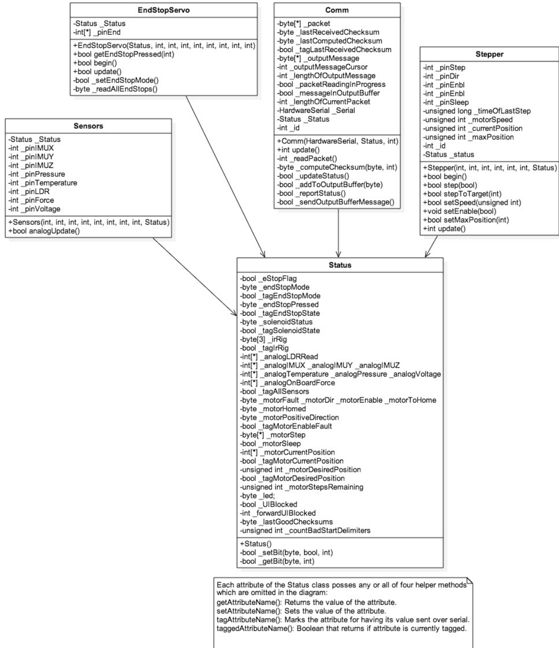
Figure 6-1: UML class diagram for Main Code V1.
