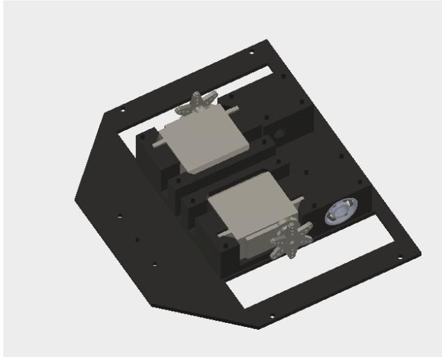
Mount the left and right supporting walls to the bottom of the robot. Push the drive axle through the support supporting walls as well as the drive axle. Add a gear and idler horn onto the wheel axle and push it through into the second bearing, aligning the gears. Mount the wheel to the wheel axle and add a drop of super glue to prevent the axle from slipping. The chassis should look like this.
