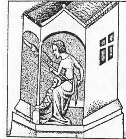
Figure 34 Woman using a spindle and long distaff. The distaff is secured in her belt. (From Singer, 1956)
