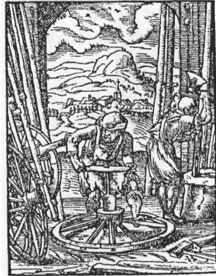
Figure 24 A Wheelwright's shop. The wheelwright in the foreground is drilling the center of the hub. (From Singer, 1956)
