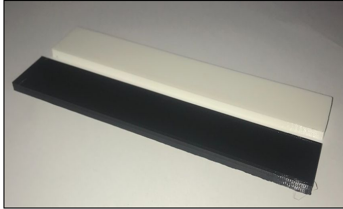
Figure 14. PLA Specimens used in Testing.
