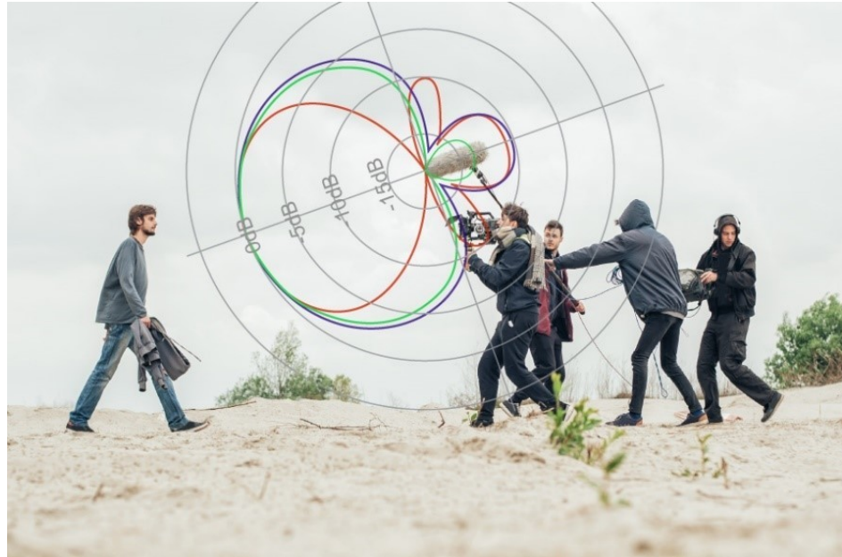
Figure 18: Example of directional pickup pattern by Azden Corp. (2018)
