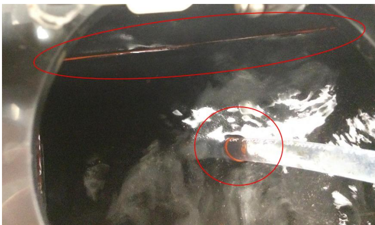
Figure 5. Dyed Oil Sticking to the Inside of the MBR
