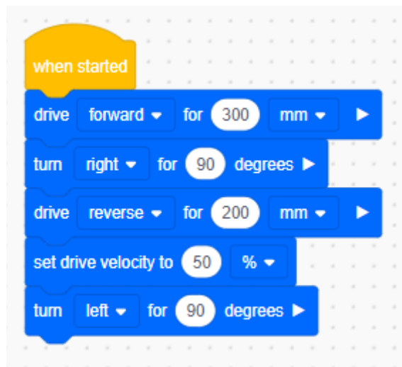
Figure 15: A basic program showing some of the Drivetrain blocks
