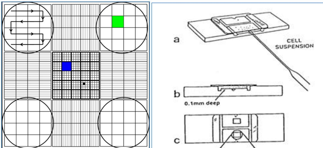
FIGURE 17: IMAGE OF HEMOCYTOMETER DEVICE (LEFT) AND 9X9 GRID (RIGHT)
