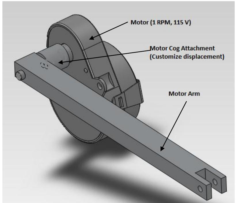
FIGURE 12: MOTOR AND CAM SYSTEM
