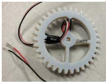
Figure 45: Gear sensor used in the final prototype
