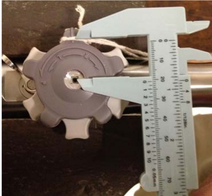
Figure 67: Measuring the distance from the center of the small knob to the string tie. String should be carefully secured at measured distance with duct tape.
