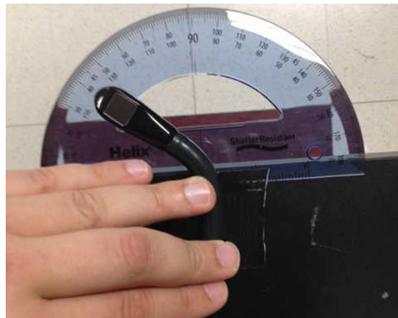
Figure 51: Displacement test of original TEE CCW yaw
