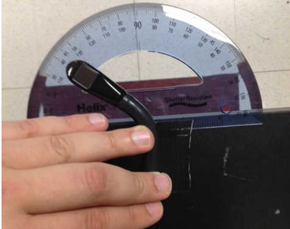
Figure 70: Displacement test of original TEE CCW yaw
