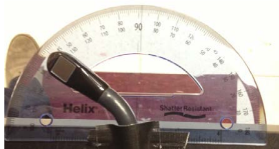
Figure 52: Displacement test of modified TEE CCW yaw
