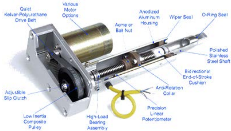
Figure 13: Traveling-nut linear actuator (The Bug)
