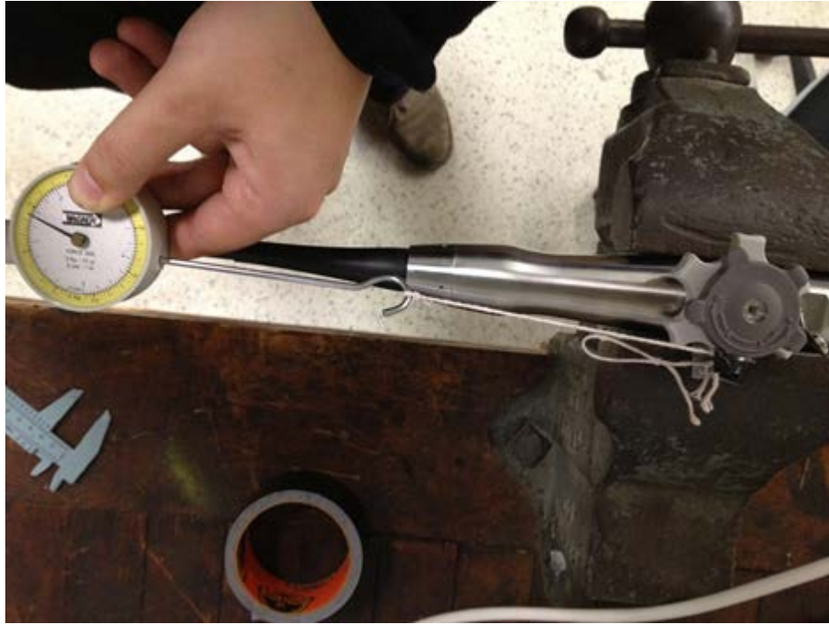
Figure 69: Illustrates measuring the safe torque value for small knob. Notice string is pulled tangentially to knob.
