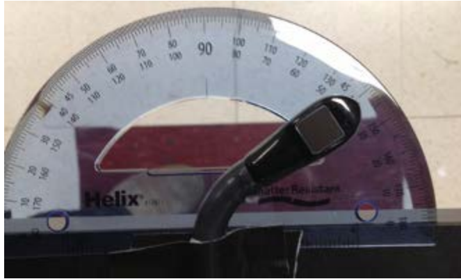
Figure 72: Displacement test of original TEE CW yaw
