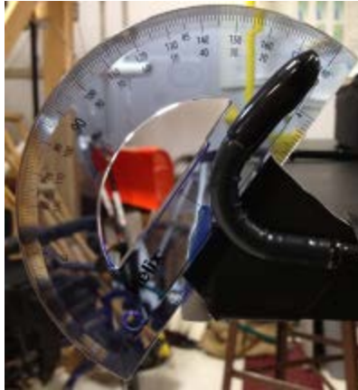
Figure 78: Displacement test of modified TEE CCW pitch
