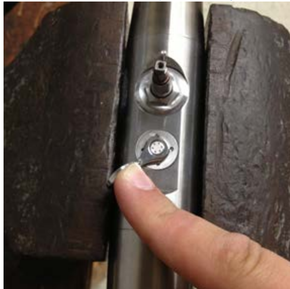
Figure 64: Illustrates the "on" position for the safety slip clutch.
