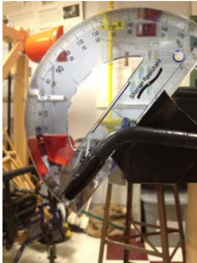
Figure 76: Displacement test of modified TEE CCW pitch
