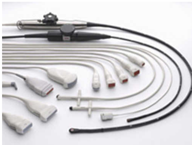
Figure 1: This image shows various TEE probes manufactured by Phillips Electronics. (Koninklijke Phillips Electronics N.V., 2012).
