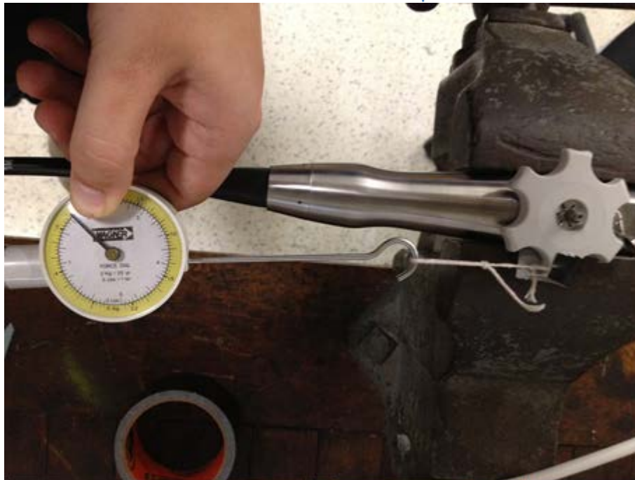
Figure 68: Illustrates measuring the safe torque value for large knob. Notice string is pulled tangentially to knob.
