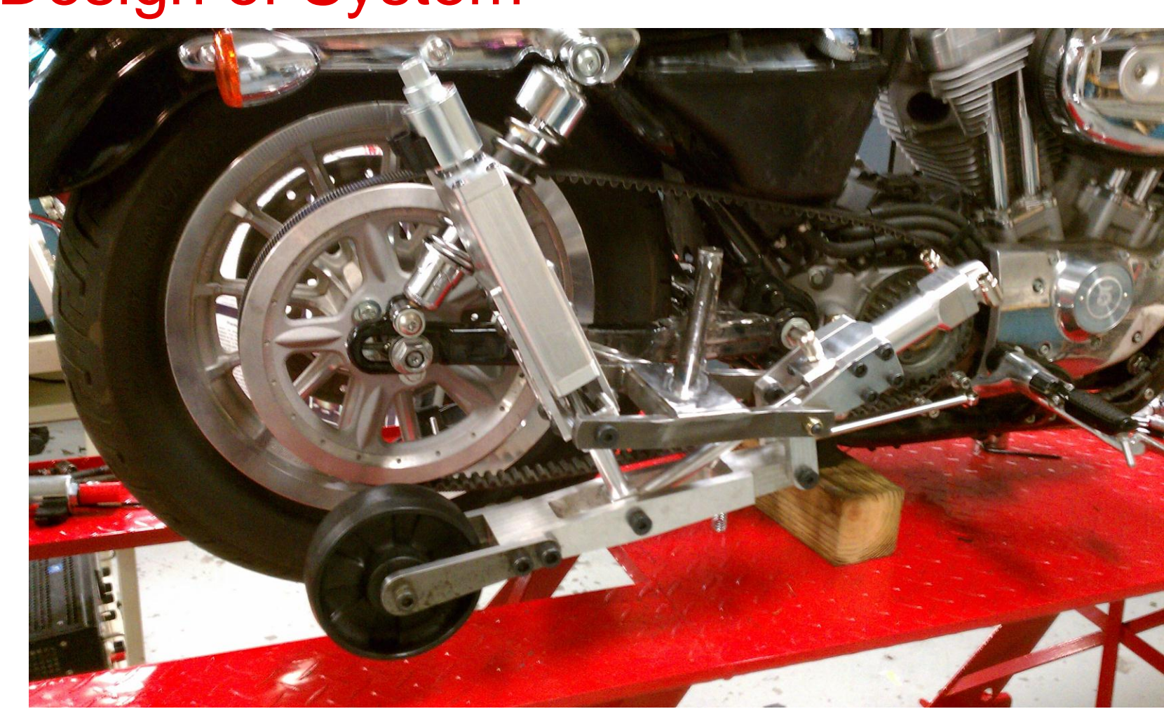
Assembled Mechanical System
