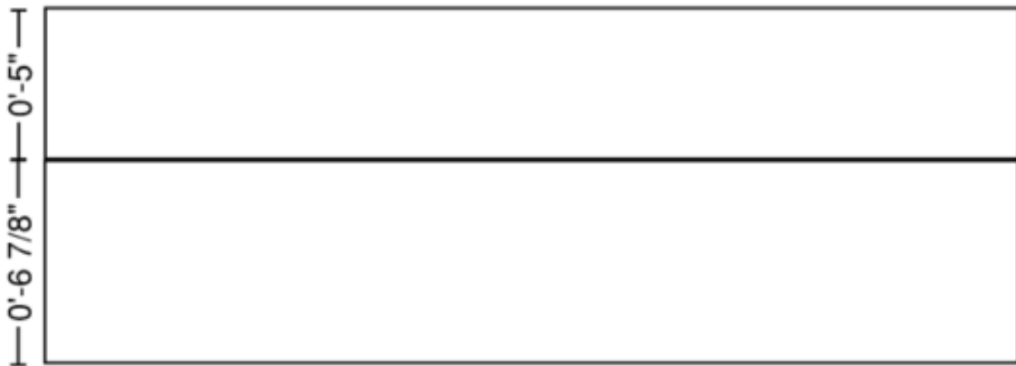
Figure 6.4. Concrete On CLT Paneling
