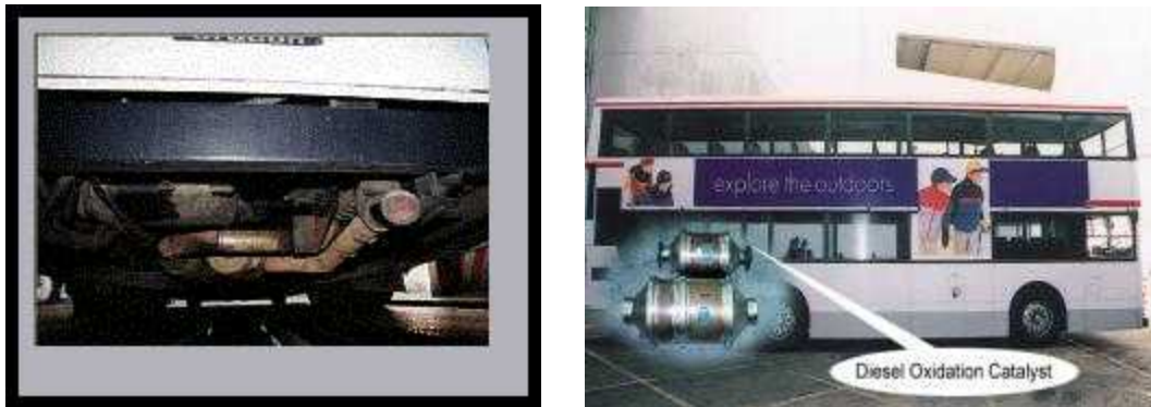
Figure 65: Position of diesel oxidation catalyst
