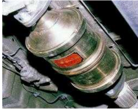
Figure 63: Particulate reduction devices for pre-Euro light diesel vehicles
