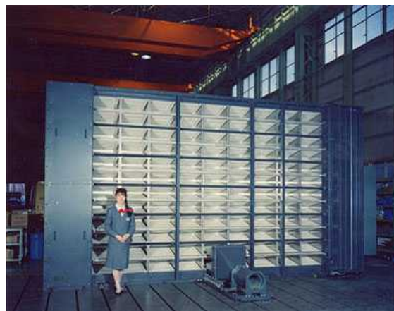
Figure 47: Smoke Soot Filter Plant
