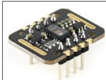
Figure 5: Image of the MAX30102 Pulse Oximeter used in the Arm Cast
