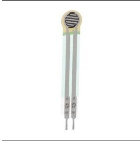
Figure 4: Image of the Strain Gauge Model used in the Arm Cast
