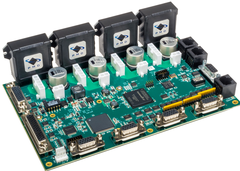
Figure 30: PMD Machine Control Board
