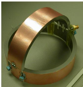
**Figure 2.9: Single Ring-Strap Coil Prototype**
