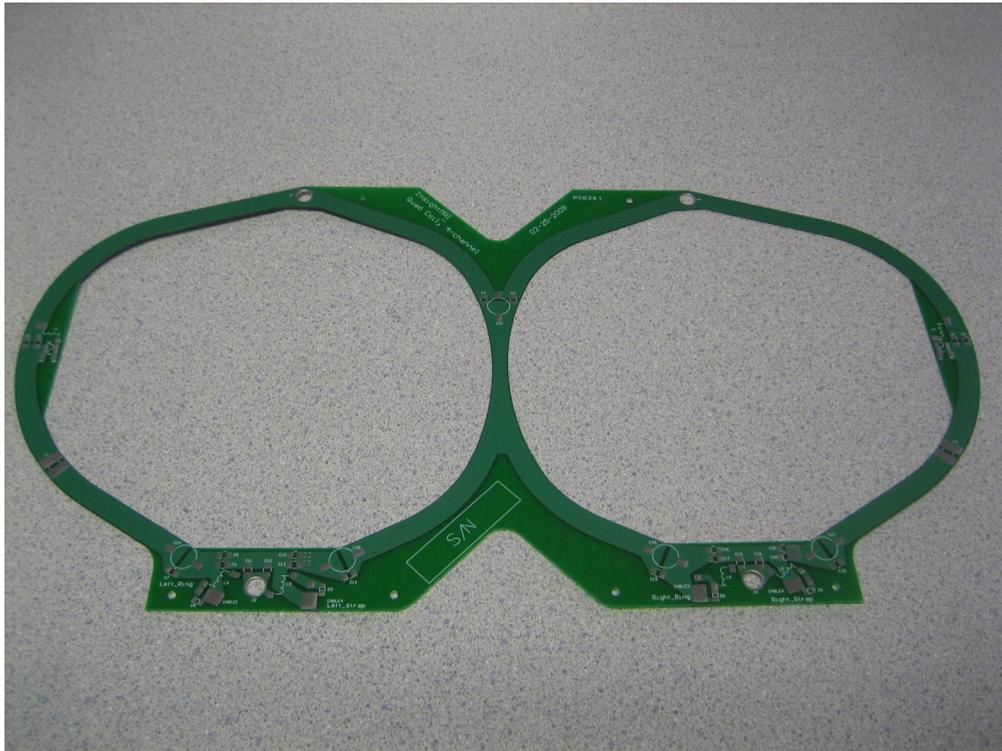
**Figure 5.3: Manufactured Main PCB**
