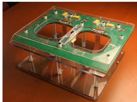
**Figure 2.10: Dual Ring-Strap Coil Prototype**
