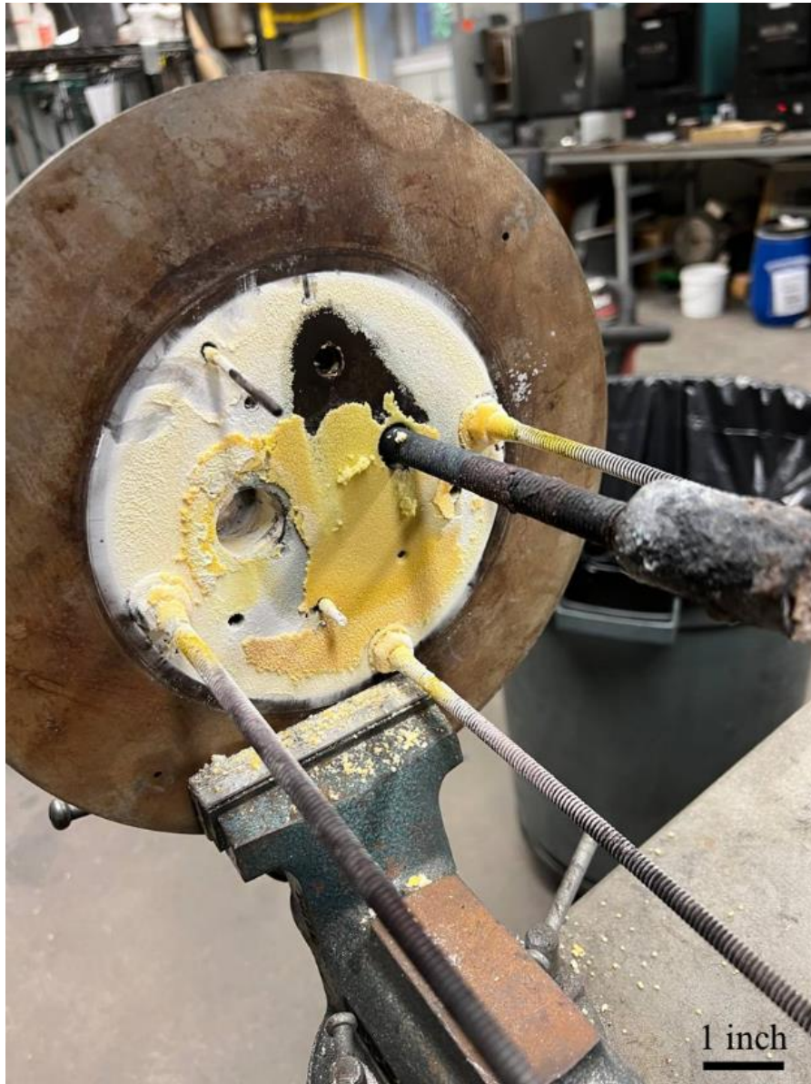
Figure 29, Furnace door from the inside after experiment 16 showing the ammonia chloride deposited around the furnace wall from inside
