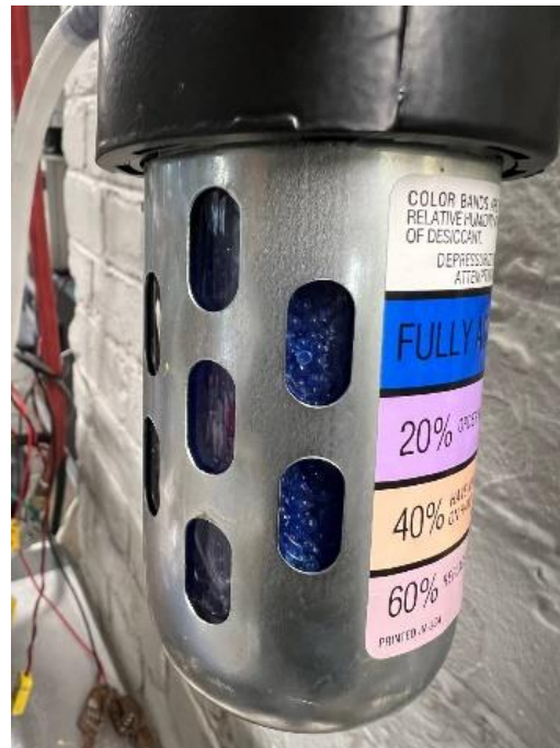
Figure 14, Desiccant air dryer used in experiment 9
