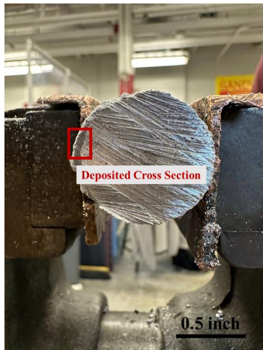
Figure 41, The Mg after recharging showing the cross section and deposited lump from experiment18
