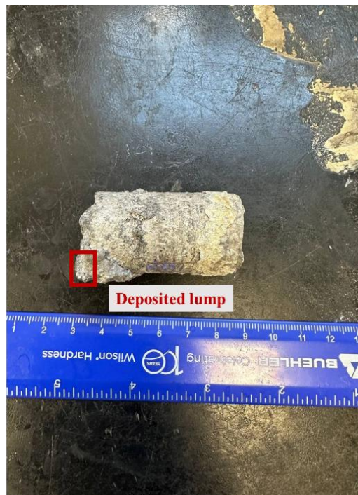
Figure 41, The Mg after recharging showing the cross section and deposited lump from experiment18
