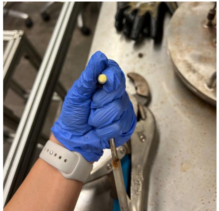
Figure 33, Right) The cage after the long discharge of experiment 17, showing the huge solidified component formed on the cold finger as well as the cathode Left) the gas outlet pipe of the furnace was blocked as a result of using ammonia chloride
