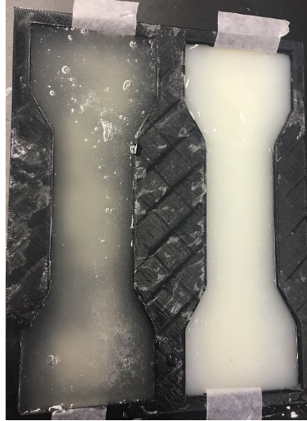
Figure 16: Agar (Left) Versus Agar and Cornstarch (Right) in Tensile Mold
