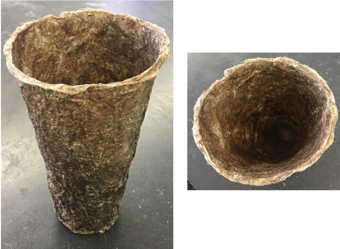
Figure 61: Dried Cup Form Before Wax is Added (Side and Top View)
