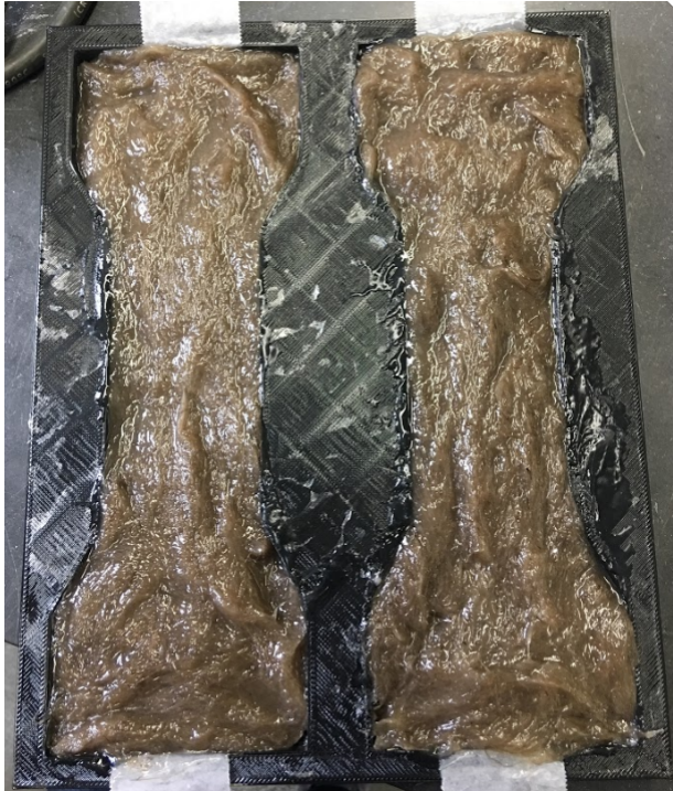
Figure 17: Tensile Strips in Mold with Agar and Hemp
