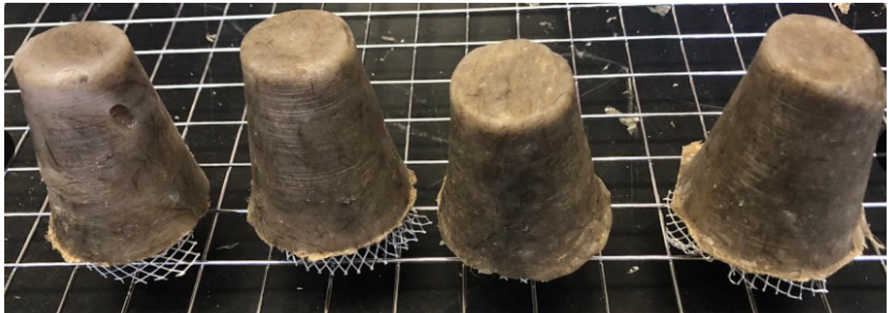
Figure 8: Cooled Hemp-Agar Pulp on Mesh Drying Mold
