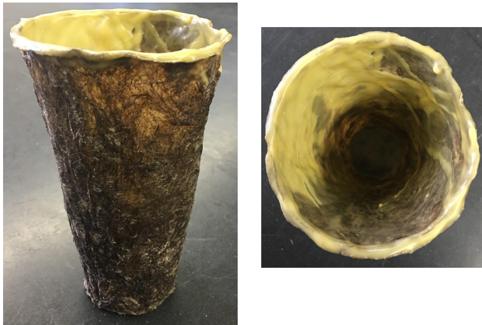
Figure 62: Final Hemp-agar Cup with Wax Coating (Side and Top View)
