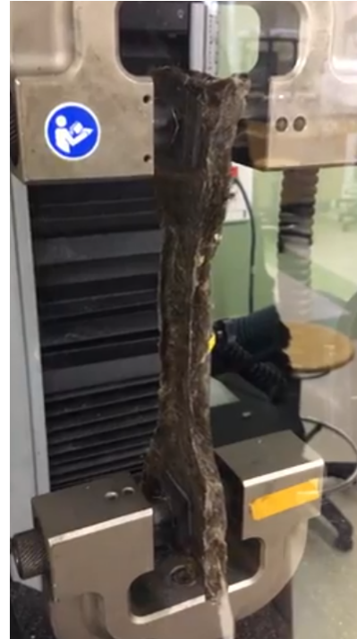
Figure 18: Agar-Hemp Strip Prior to Testing in Instron 5544
