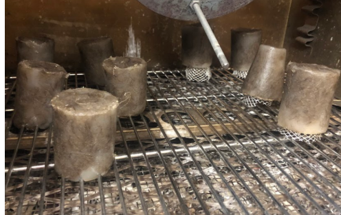
Figure 9: Hemp-Agar Cup Samples in Convection Oven.
