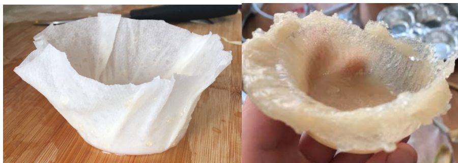
Figure 11: Glue Coated Paper Towel (Left) and Rudimentary Gelatin Cup (Right)
