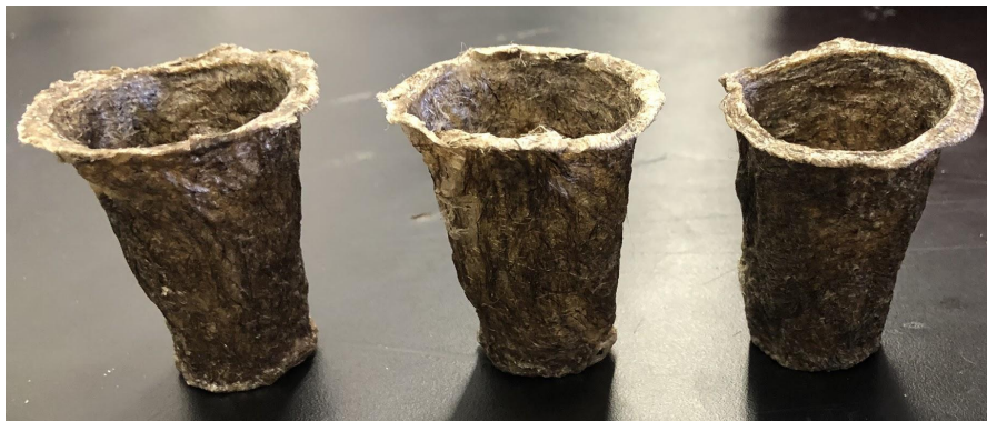
Figure 36: Dried Cups from Draft Angle PLA Mold and Wire Mesh Support
