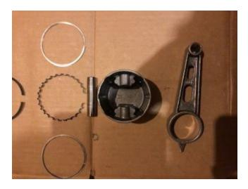
Figure 21, Connecting Rods, Piston Heads, and Piston Rings
