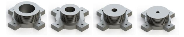
Figure 51, Cylinder Chamber Stages 1 (left) through 4 (right)
