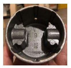
Figure 22, Piston Bottom View
