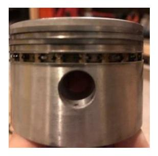
Figure 24, Piston Ring Assembly
