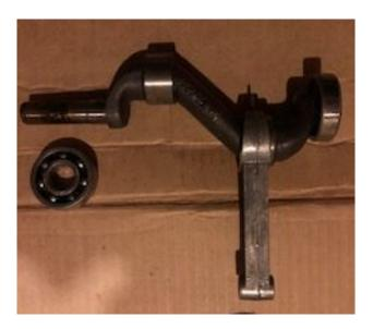
Figure 25, Crankshaft Assembly
